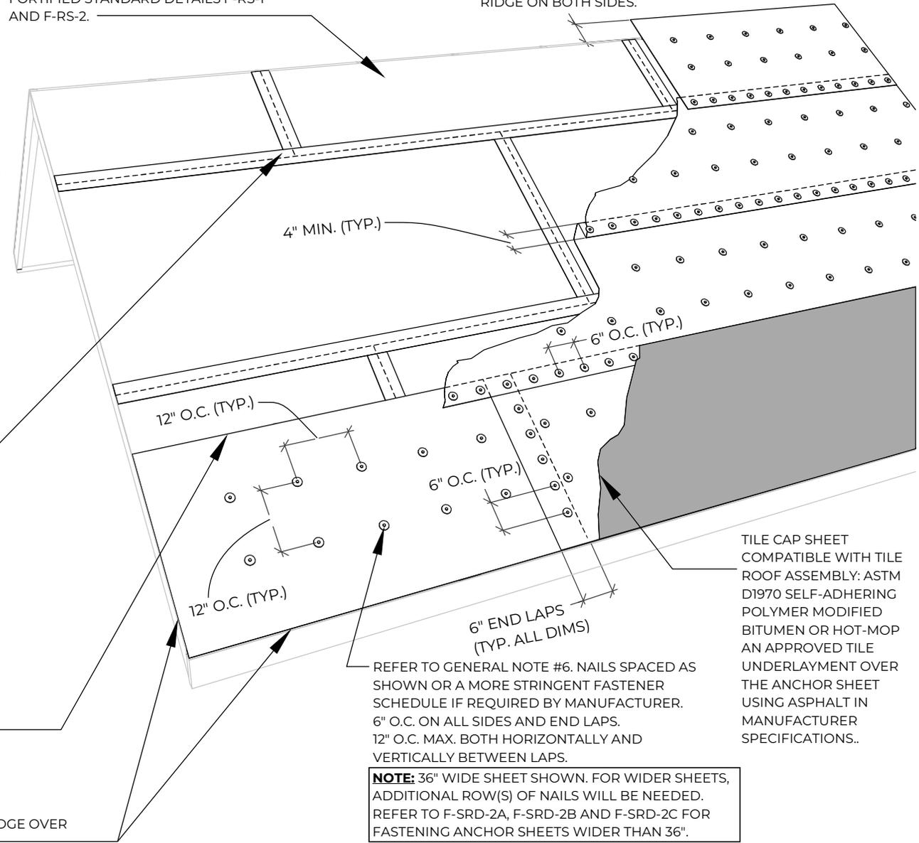
FLASHING TAPE AT ALL PANEL SEAMS FULLY ADHERED W/ NO WRINKLES OR VOIDS USING ROLLER.
