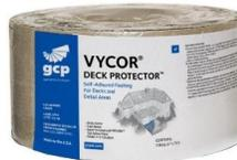
**Vycor Deck Protector** helps reduce corrosion of galvanized metal connectors. It is installed between the connector and the pressure-treated wood and acts as a barrier layer to break the electric circuit and thus helps reduce corrosion.
